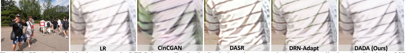
Figure 8. SR results of video images on the REDS dataset. For Real → Real adaptation across devices, only qualitative visualizations of SR results are provided. Because only HR video images are realistic data, we take those HR video images in REDS as the target LR images to verify the proposed model.
